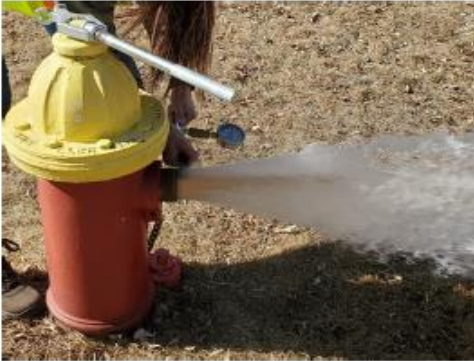
Figure 13. Example Pitot Tube Measurement
